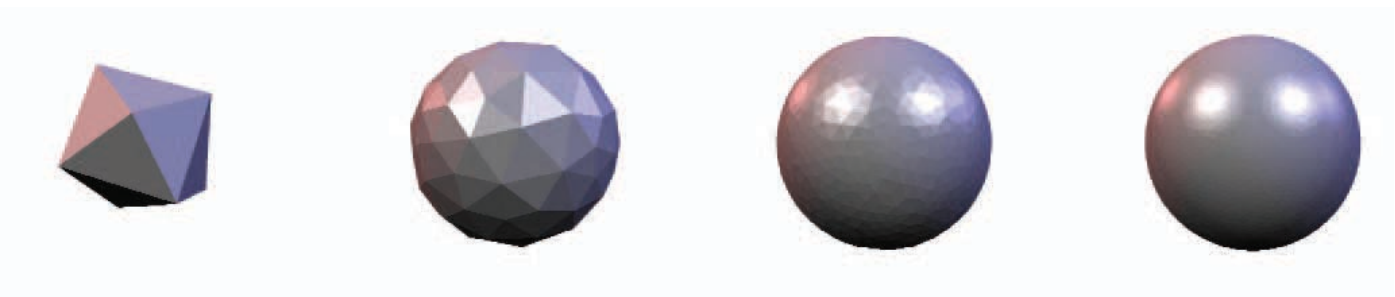
Figure 1. A sphere reconstructed from an implicit surface. The polygonal meshes have 10, 100, 1K and 5K vertices, corresponding.
