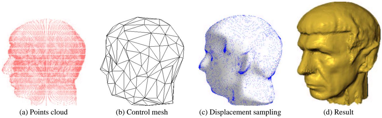
**Figure 11. Reconstruction process and result (spock model)**
